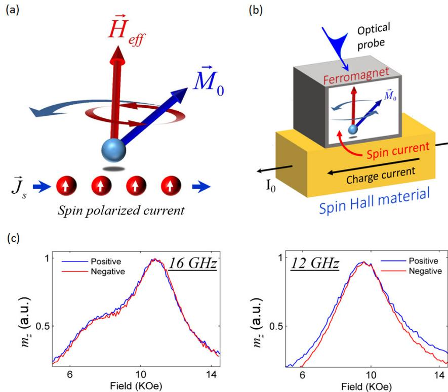
**Enhanced sensitivity for measurement of proximate spin currents. (a) Measurement concept. (b) Experimental realization. Spin current is generated in Pt film by the spin Hall effect and injected into a Co|Ni|Co trilayer. (c) Measured resonance linewidth in the trilayer for 16 GHz (left) and 12 GHz (right) for positive and negative current polarity in the Pt. The torque generated by the spin current is sensed only when the potential barrier is shallow (12 GHz).**
